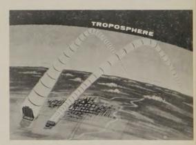
TROPOSPHERIC SCATTER SYSTEM designed and developed by General Electric accomplishes over-the-horizon communications by beaming and reflecting from the troposphere. Defense Systems Department engineers are now applying this concept to development of advanced communications systems.
