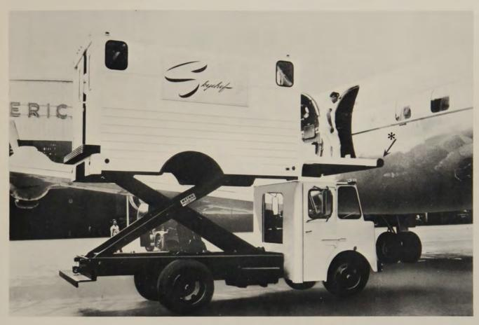
\*Safety device—platform bumper against plane, sensitized. If plane settles during loading (flat tire, etc.) hoist automatically lowers self to prevent damage to plane or hoist.
